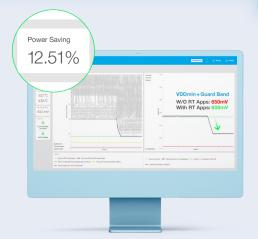
AVS Pro safely reduces voltage guard bands, enabling substantial power reduction
